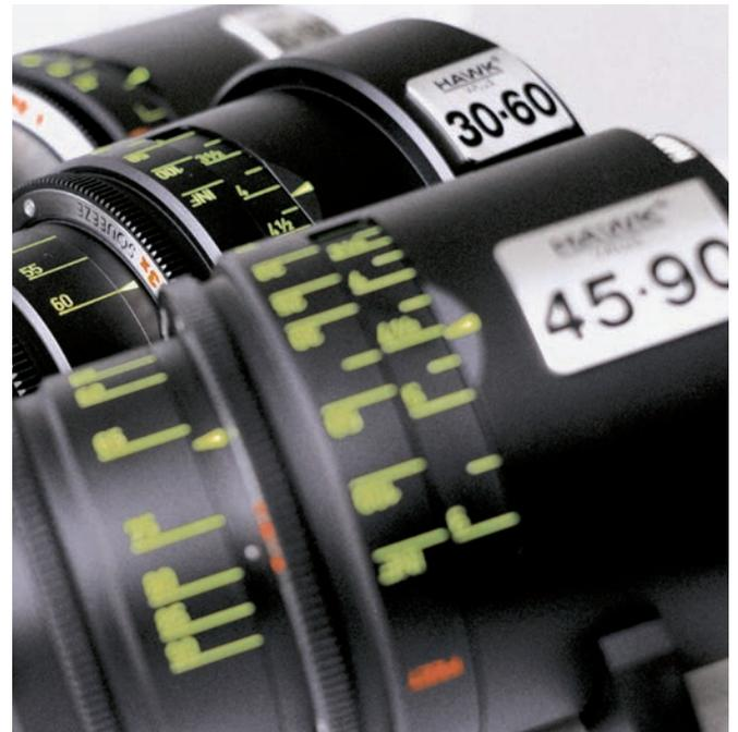
*Hawk 1.3x Anamorphic Lenses can be used on all modern digital and film cameras. The unique squeezing factor of 1.30x makes it possible to use nearly the entire sensor area of a 16:9 digital camera and achieve the popular widescreen 1:2.40 release format. Furthermore the lenses can stretch the 4:3 negative/sensor area to 1:78 for 16:9 HDTV release. No matter which format you ultimately decide on – the new Hawk 1.3x Anamorphics use 33% more sensor/negative compared to standard spherical lenses.*
